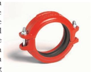
adjustment also forces the key sections into opposed contact on the inside and outside groove edges, pushing the joint to its maximum pipe end separation during assembly. These products can be considered to have system behaviour characteristics similar to those of welded or flanged systems, in that all piping remains in strict alignment and is not subject to deflections during operation and electrical continuity is also maintained.
